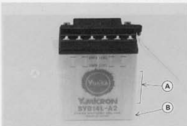
A. Sulfation here B. Sediment here
