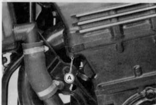
A. Cylinder Head Bolt (6 mm)
