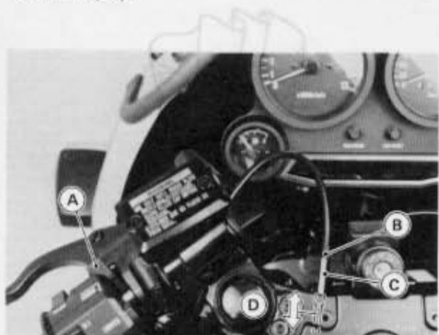
A. Choke Lever C. Adjusting Nut B. Locknut D. Play
