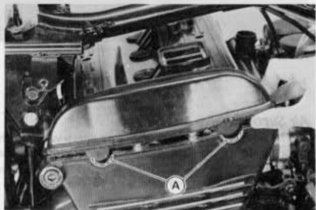
A. Apply silicone sealant here.
