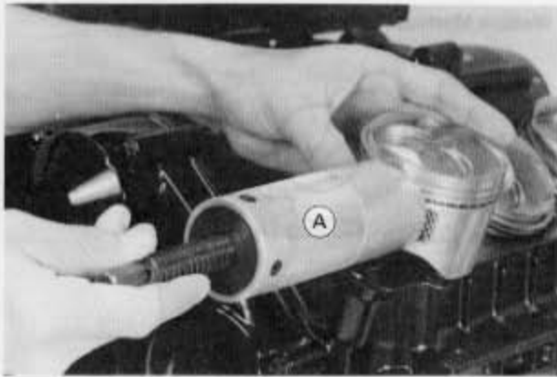
A. Piston Pin Puller Assembly: 57001-910
